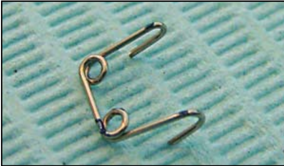
Fig. 3 Legs of spring bent into J-hooks and excess wire cut off.
